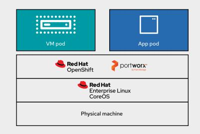
Figure 2. The joint solution simultaneously supports both VM and application pods
